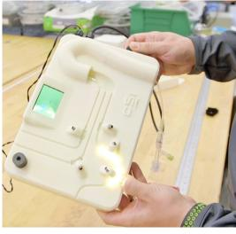
Medical device developers like CSI use 3D printed models that mimic a range of tissues, incorporate access points, sensors and blood-flow simulation. These anatomical models replicate hard plaque and pliable, durable vessels without the need for biohazard controls. The digital model inventory also makes it easy to print more as needed anytime, anywhere.
