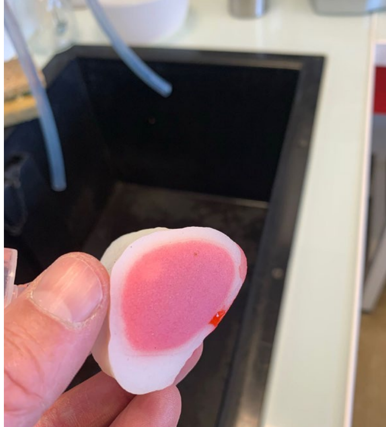
The J5 MediJet’s multi-material multi-color 3D printing capability enables the production of ultra-realistic models for pre-surgery preparation and training
