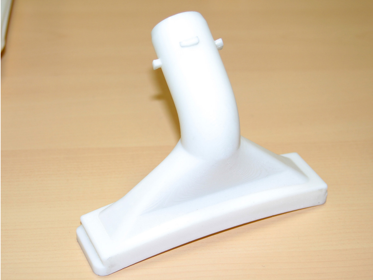
3D printed vacuum nozzle for the removal of any contaminating particles, produced using the Fortus 450mc 3D Printer.
